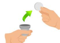
1. Remove the outlet head and **dispose of the filter disc**. A new filter disc is inserted daily at the start of operation.
